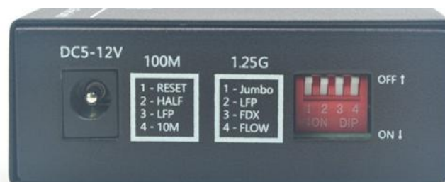
Figure 4 : DIP switch for 10/100/1000
